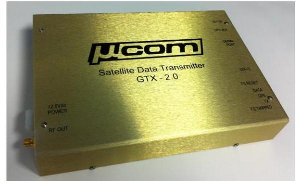
The Microcom GTX-2.0 Satellite Transmitter and Data Collector is certified for 100, 300, and 1200 BPS operation on GOES DCS for Self Timed and Random operating modes. (Certificate # xxxxx). Operation on GMS is Self Timed. On METEOSAT it is Self Timed on the International channels. User selectable GOES, SCD, or ARGOS operation.
