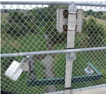
River Level from Bridge
