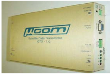
Microcom GTX Satellite Transmitter
