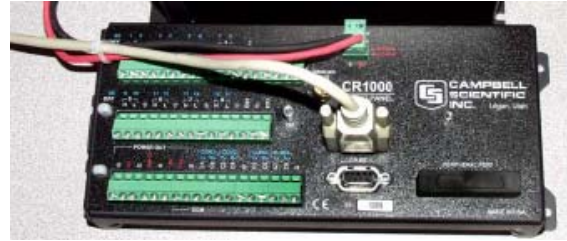
Campbell Scientific Programmable Data Logger
